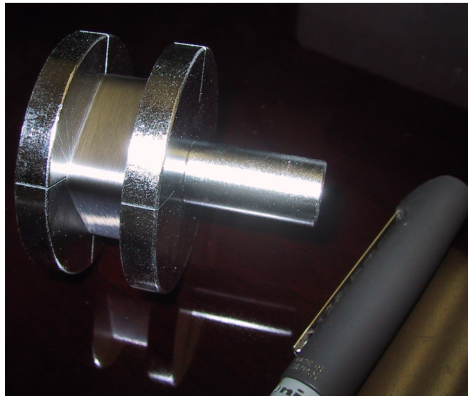
Figure 6. Early version of moly spool used for winding tungsten wire
