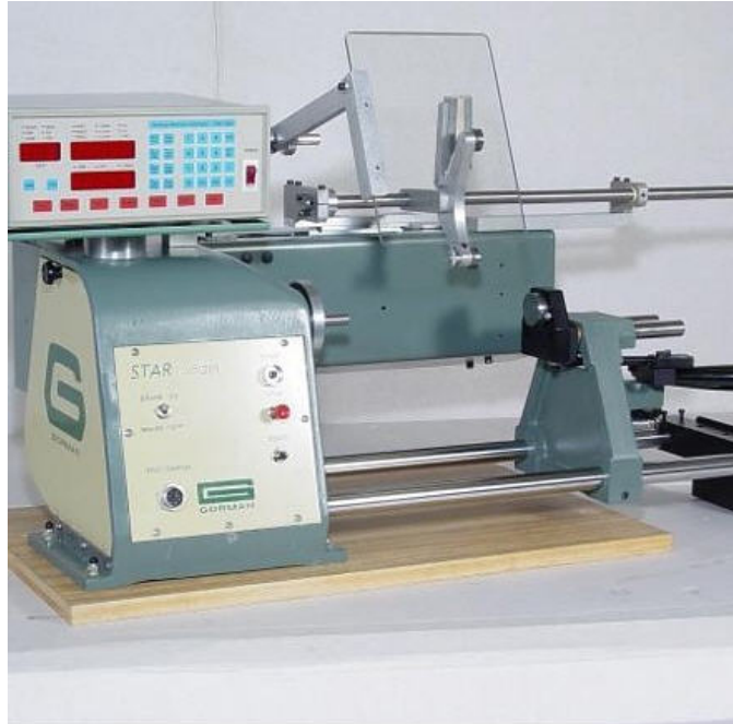
Figure 5. Machine for winding 20 micron diameter tungsten wire for controlled porosity material
