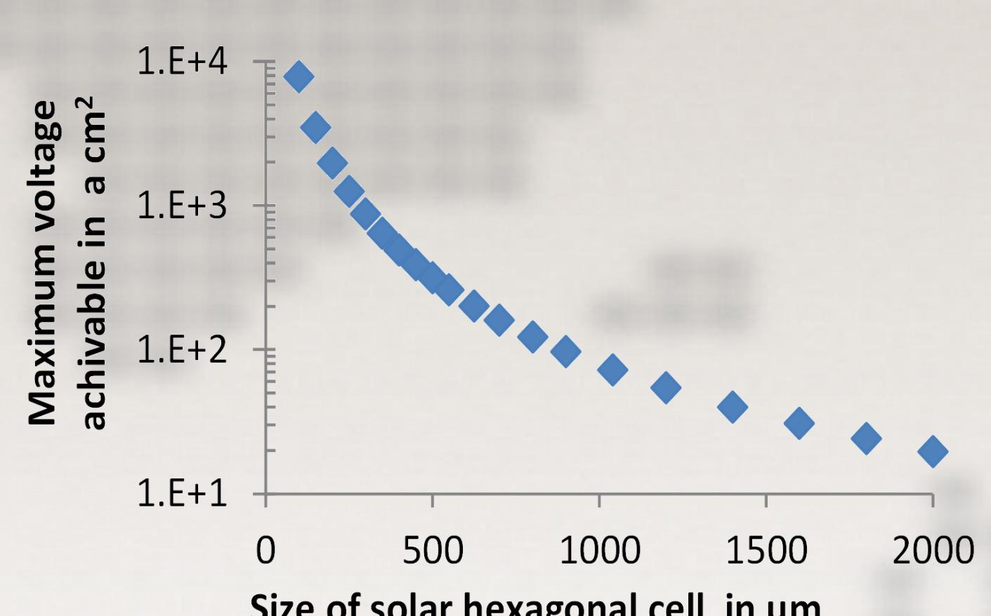
Small cells can achieve high voltages in very small area. The graph shows the maximum voltage as a function of cell diameter measured from corner to corner of the hexagonal shape cell.
