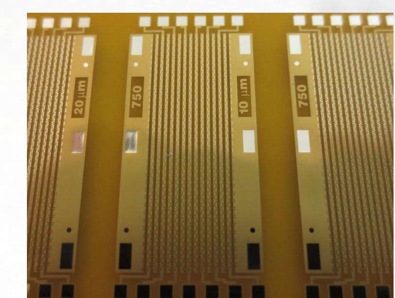
A patterned flex circuit that matches the position of the solder bumps was fabricated to receive the cells.
