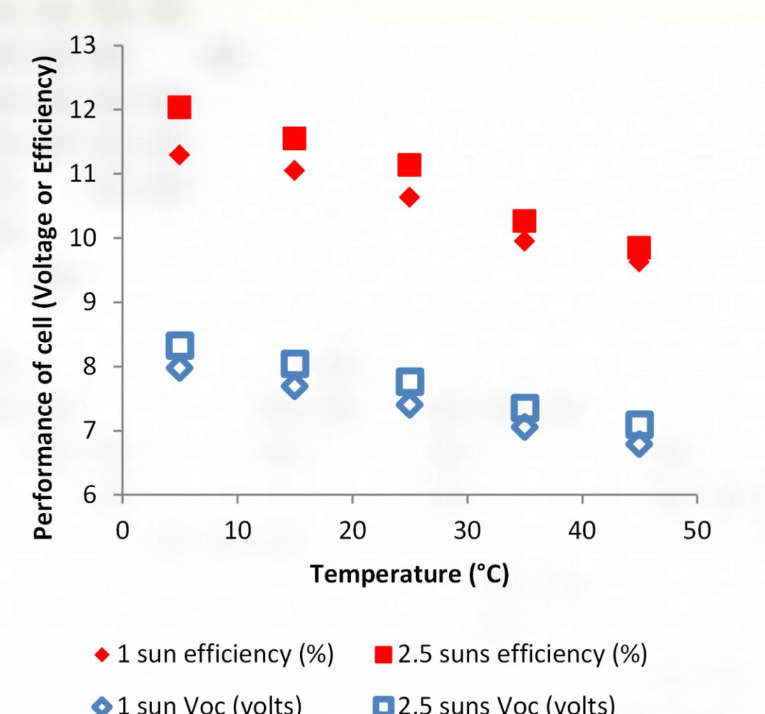
A temperature dependence study shows that the micro cells behave as macro sized solar cells. Voc slope is 2.14V/°C for each cell. The performance shown is for a module with nominal efficiency of 10.7%.
