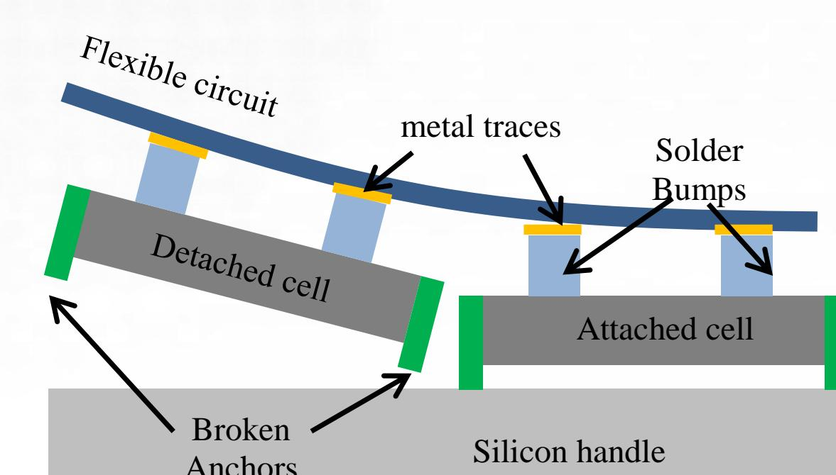
The flex circuit is physically pulled and all the anchors attaching the cells to the handle wafer are broken, thus completing the transfer of the cells to the flex circuit.
