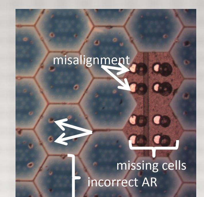
Zoomed image of cells that produced a 4.9% efficient mini-module using 500  $\mu\text{m}$  cells.
