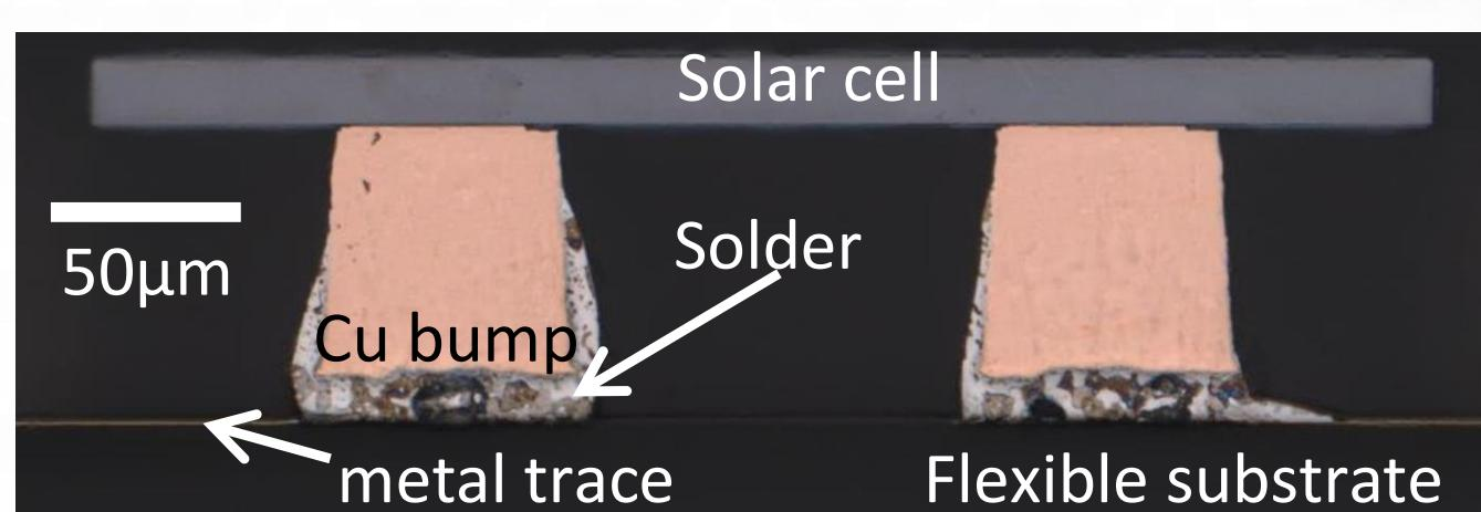
Once the solder wets the receiving substrate, the temperature is lowered so the solder can harden. After the stack is cooled below the melting temperature of the solder, the cells are electrically and mechanically connected to the flexible circuit
