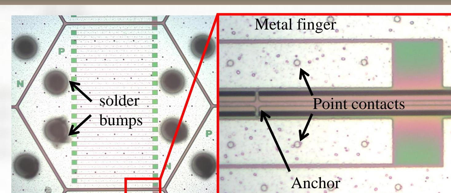
The fabricated cells have interdigitated back point contacts. At the end of the fabrication, the cell is fully functional and attached to the handle substrate by thin tethers.
