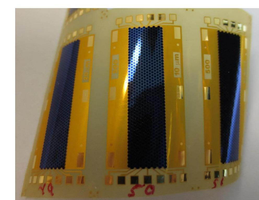
Solar mini-module operating while being flexed. Multiple series parallel connections keep the voltage unchanged while flexed.
