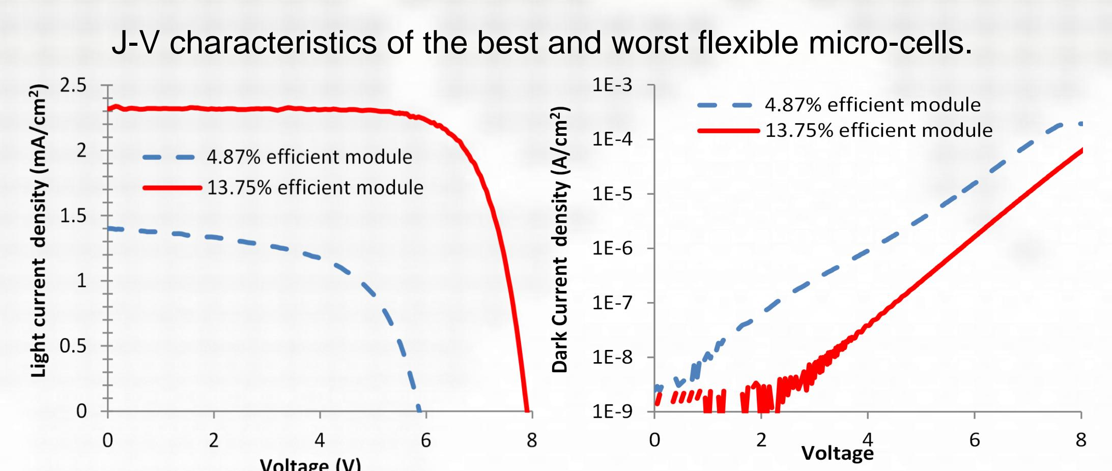
The light current and voltage were limited due to missing cells and tear offs in the cells.
