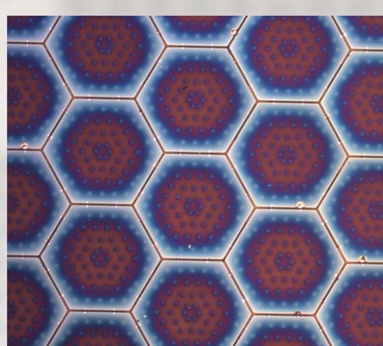
Zoomed image of cells that produced a 13.7% efficient mini-module using 720  $\mu\text{m}$  cells.
