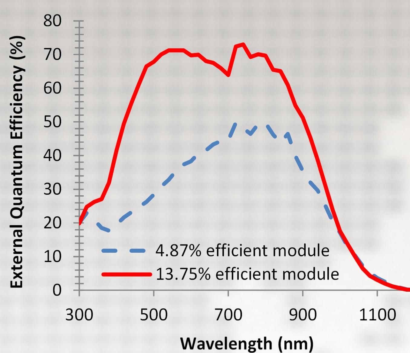
EQE measurements show that tear offs produce high surface recombination velocity that trap carriers with high energy.
