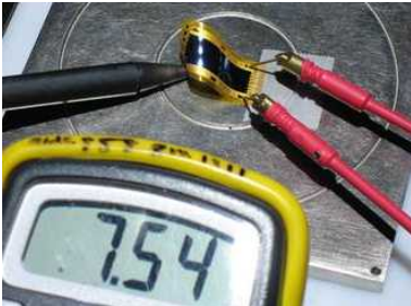
Fig. 7. Voltage measurement of the mini-module while being flexed.
