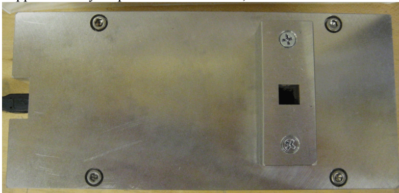
Figure 2: Shield and Collimator Assembly for Enrichment Measurements
