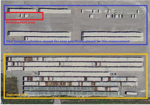
Fig. 2. The measurement area (red box) is shown in relation to a source of background (yellow box); other cylinders within the blue box are new, unfilled cylinders and thus do not contribute to the neutron background.
