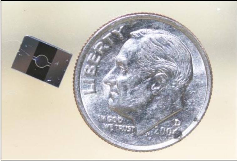
Uncoated NPD device (cantilever device) next to a dime.
