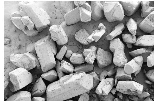
HMX003 Powder File= 003-Pow_2000um-2.tif 100 µm Mag = 69 X WD = 4.5 mm Date :18 Apr 2013 Width = 2.023 mm Stage at T = 5.0 ° Ref Mag > Polaroid 4x5 EHT = 1.50 kV Signal A = SE2 Chamber = 4.68e-005 Pa
