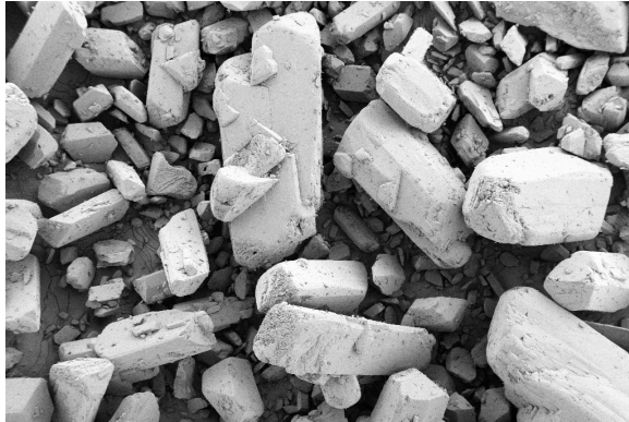
HMX001 Powder File= 001-Pow_2000um-2.tif 100 µm Mag = 60 X WD = 4.7 mm Date :18 Apr 2013 Width = 1.989 mm Stage at T = 5.0 ° Ref Mag > Polaroid 4x5 EHT = 1.50 kV Signal A = SE2 Chamber = 4.76e-005 Pa
