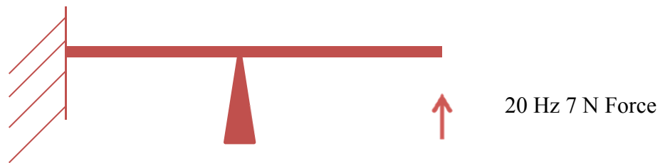
Figure 9 – Schematic of CSLDV test setup
