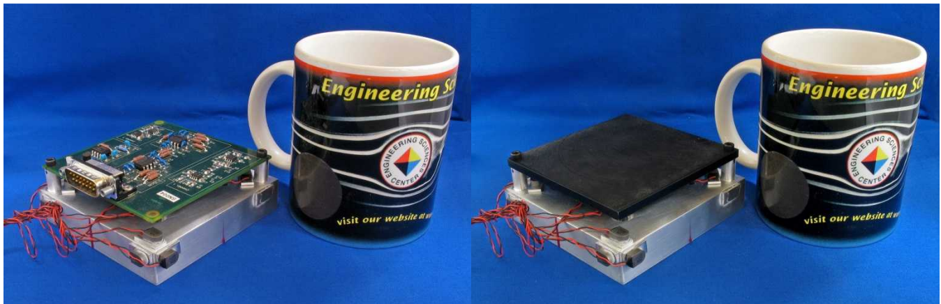
Figure 1 - Circuit Board and Fixture (Left), Truth Plate and Fixture (Right)
