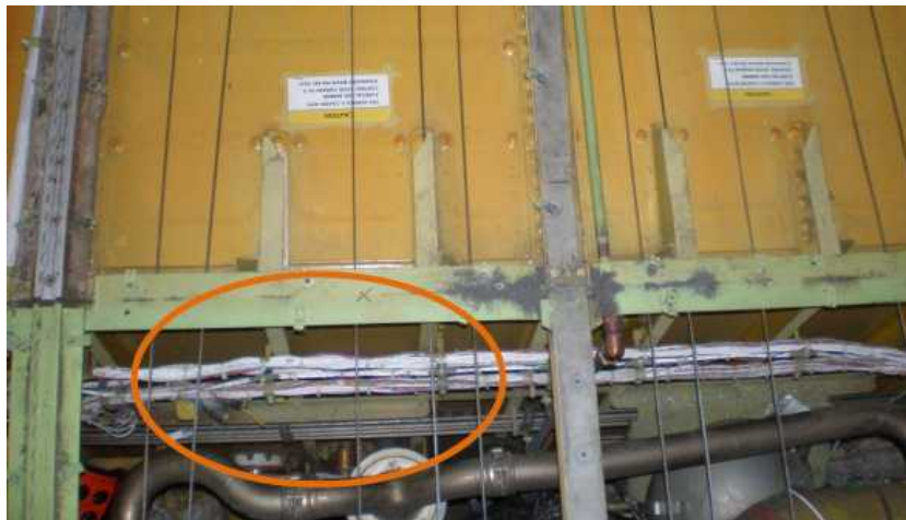
CVM Sensor on 737NG Wing Box Fitting and Top View of SLS Mount Location
