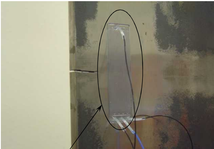
CVM Sensor Adjacent to Crack Initiation Site
