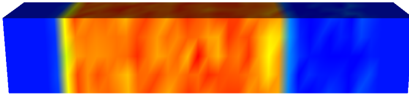
Compressive stress field for an atomic simulation of shock loading
