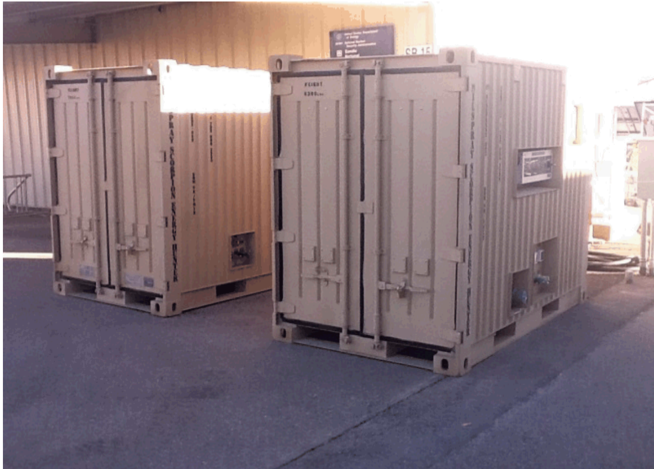
Milspray Scorpion: 15kW - 79kWh - VRLA Batteries
