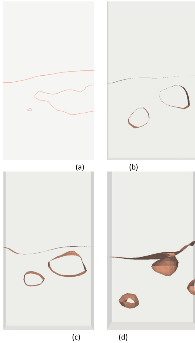
Figure 13. Transient snapshots of bubble behavior for different bed thicknesses (iso-surface of voidage of 0.75): (a) t/d_p=1, 2D ; (b) t/d_p=10 ; (c) t/d_p=20 ; (d) t/d_p=40 .
