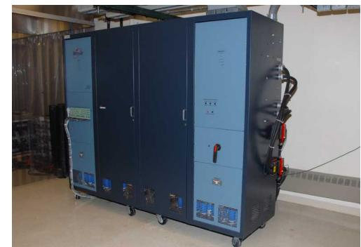
**72 V 1000 A Bitrode (2 Parallel Channels)**
