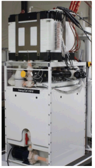
EnergyCell Beta Test: 4 kW, 23.5 kWh
