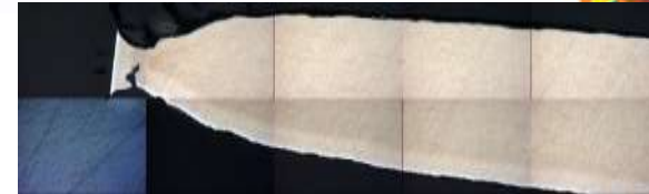
Tantalum tensile void sample
