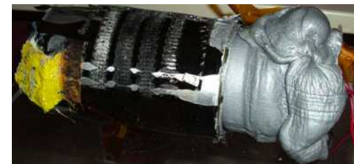
Image of failed electrolytic capacitor after high temperature operation courtesy of Jack Flicker, SNL
