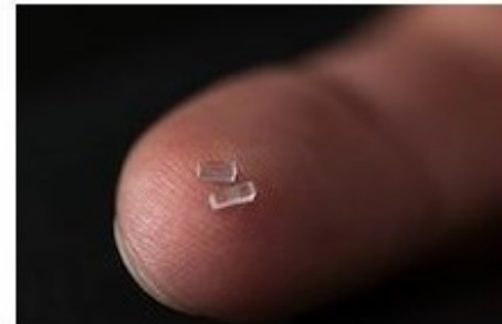
Nanofabricated chips of fused silica just 3 millimeters long were used to accelerate electrons at a rate 10 times higher than conventional particle accelerator technology. (Brad Plummer/SLAC)
