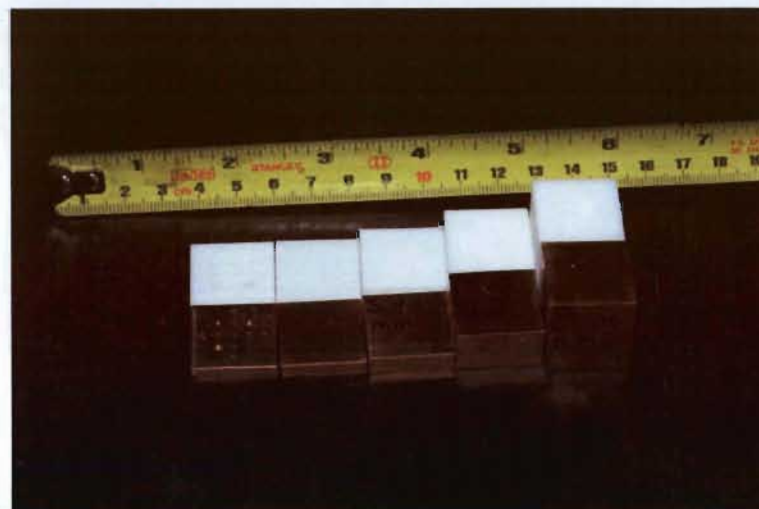
Density resolution objects (Cu and Teflon)
