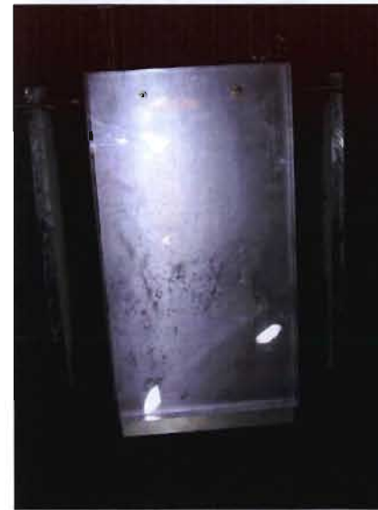
Armor plates staged around can on shot stand mounted from top door
