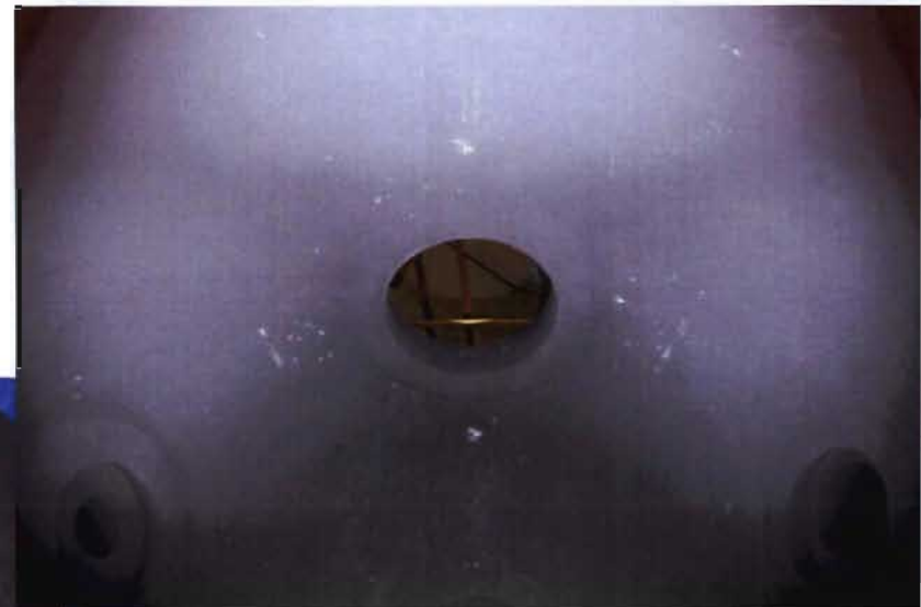
Post-shot: Damage to area around top port of vessel
