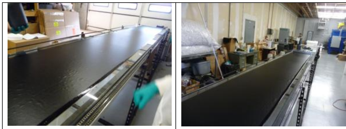
Figure 47. Diffusion layer Drying Table with high temperature baking oven in the background (right hand side photo background).
