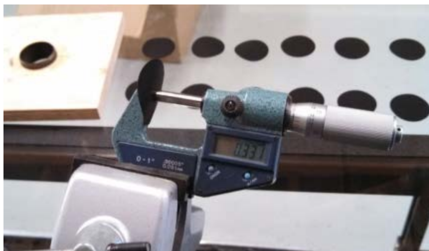
Figure 48. The thickness of NuVant's GDL circular coupons is measured with a high precision digital micrometer
