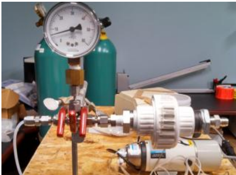
Figure 51. Gurley type device to determine the permeability of GDLs
