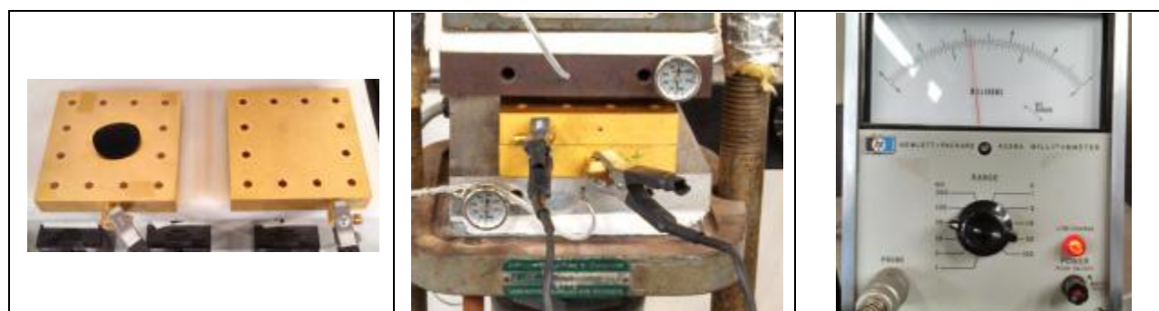
Figure 49. Apparatus for measuring the electrical resistance of NuVant's GDLs
