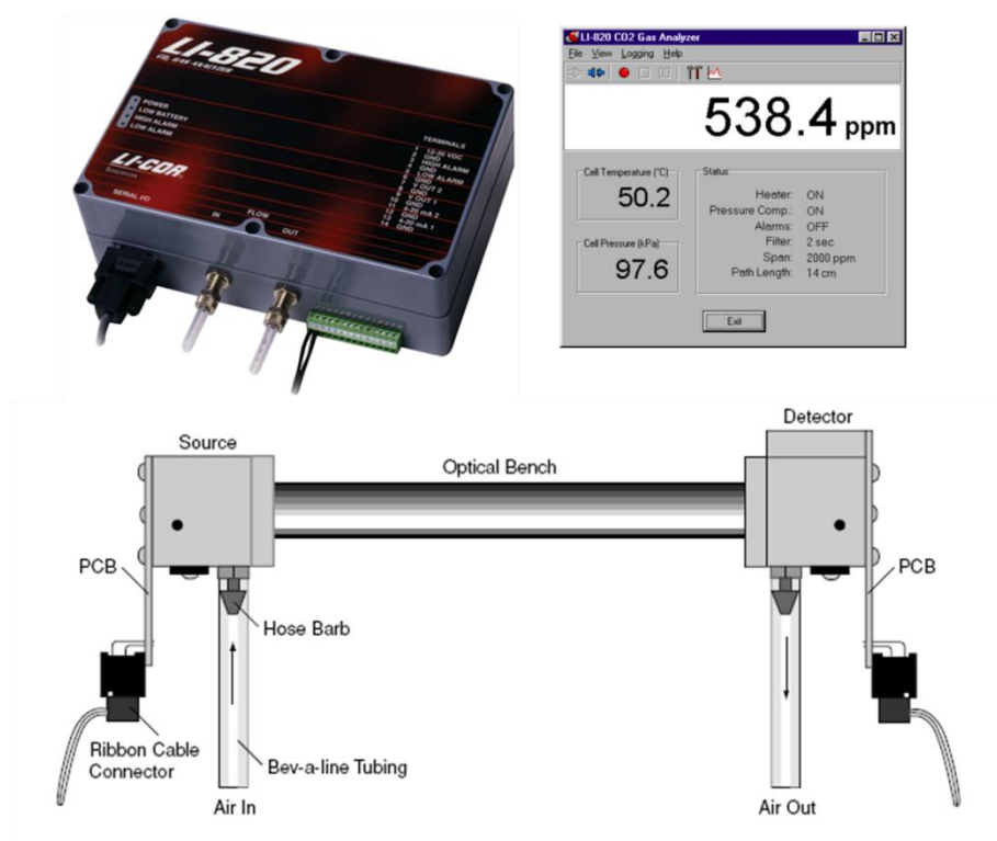
Figure 3.4 Non-dispersive infrared (NDIR) CO 2 analyzer.
