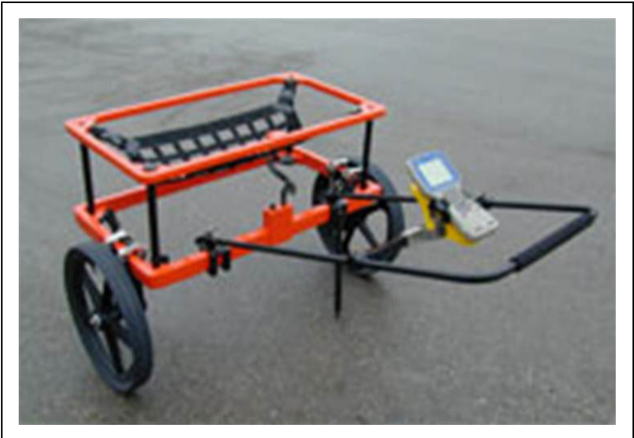
Figure G.1-2 Photo of the EM61-MK2A with Wheels Supporting Coils
