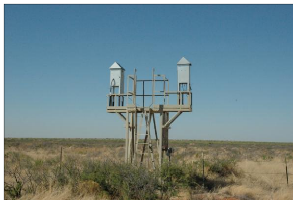
Figure 5.2 High Volume Air sampler for TSP Monitoring around the WIPP Site
