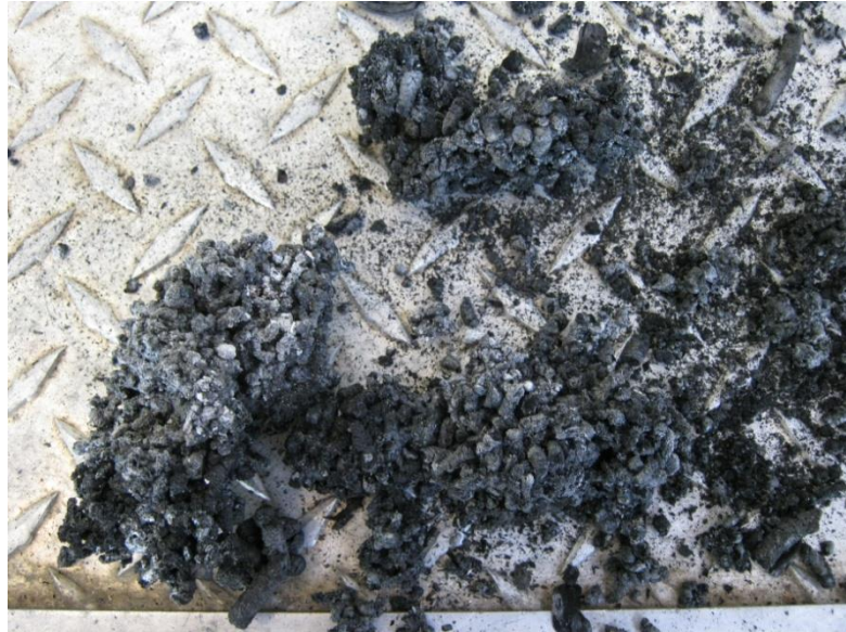
Figure K-2: Few, small switchgrass pellet clinkers
