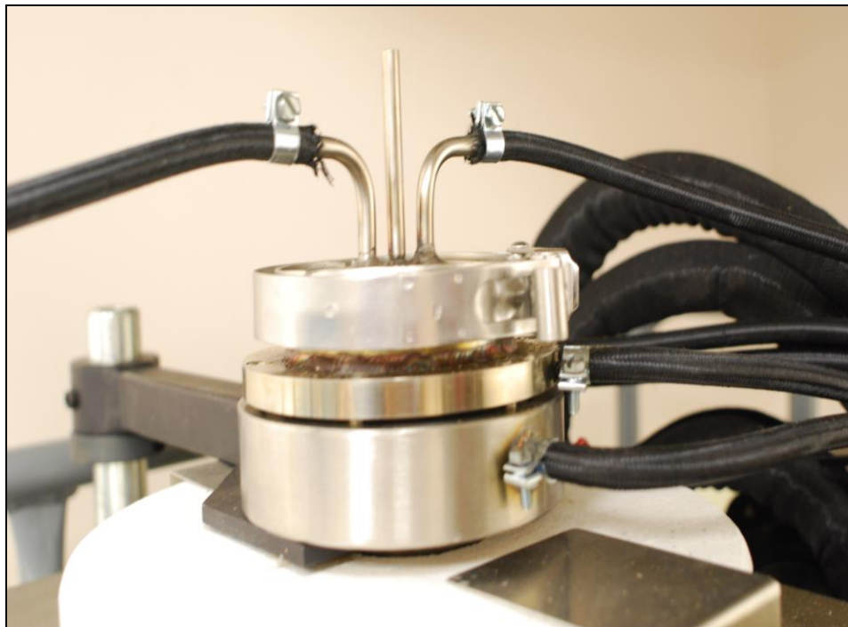
Figure E-10: Stainless steel injection nozzle shown atop retort and connected to cooling water
