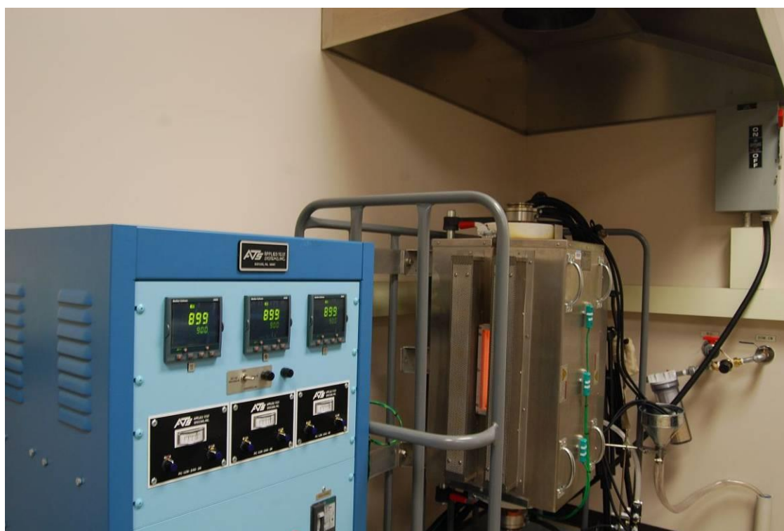
Figure E-7: The furnace shown here operating at 900°C. The controller shows the temperature in the three zones. One of the windows in the furnace is seen. The black tubes to the right of the furnace are part of the water cooling for the flanges.
