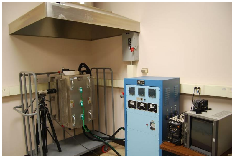
Figure E-1. The Wilmore laboratory set up is shown. The furnace is mounted to the open cage cart. The blue electrical cabinet is the controller: the three displays are for the independent furnace zones. An existing high speed CCD camera is also shown.
