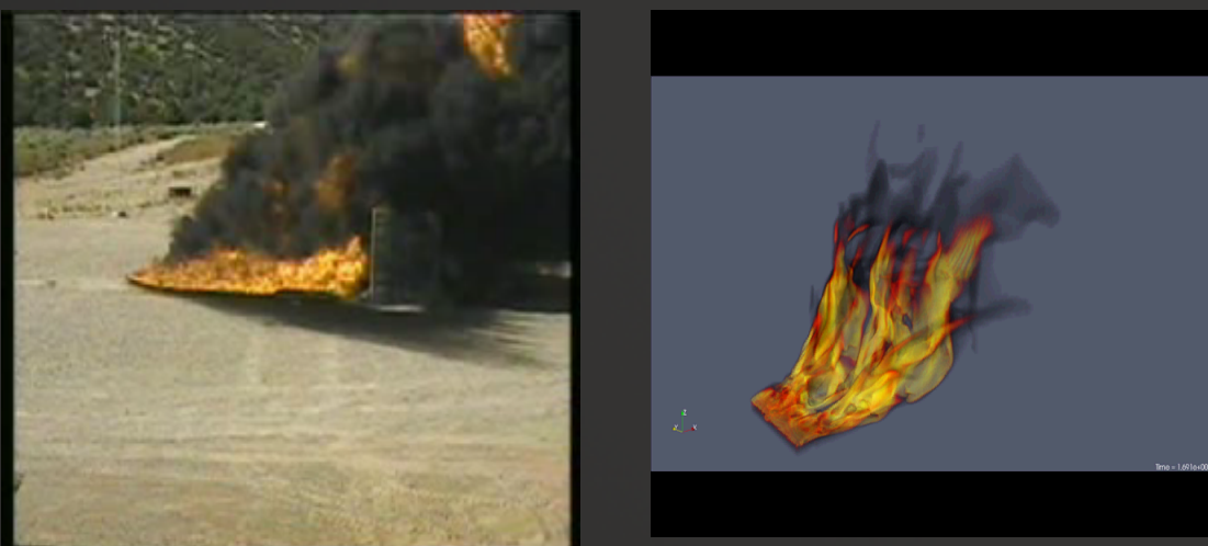
Hydrocarbon JP-8 pool fire: experiment on left, simulation on right
