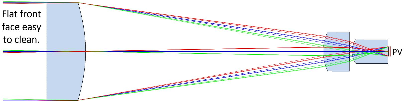
The lens arrays will be diamond-turned in Zeonex E48R. All lenses are plano-convex and aspheric.
