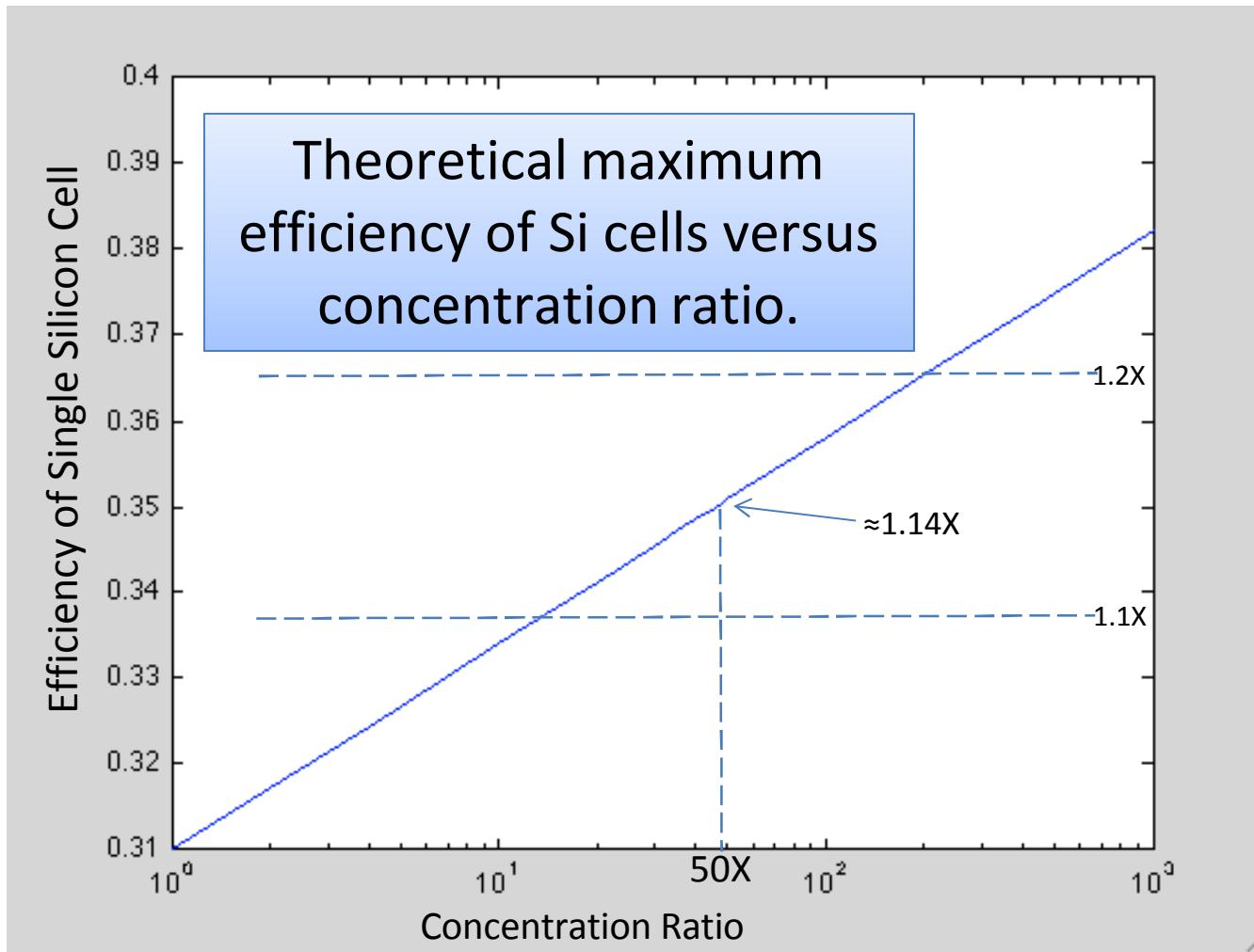
This is entirely due to the device voltage increasing with more current, in this case from 0.77V to 0.94V. This was calculated with AM1.5 spectrum.
