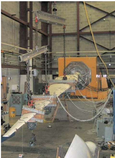
Figure 7. CX-100 blade in test fixture.
