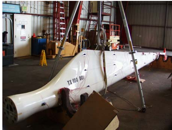
Figure 5. Single strap suspension configuration.
