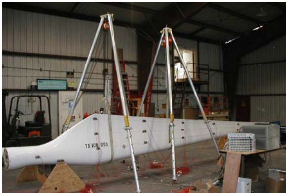
Figure 4. Double strap suspension configuration.
