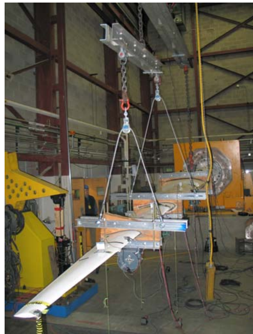
Figure 8. TX-100 blade in test fixture.
