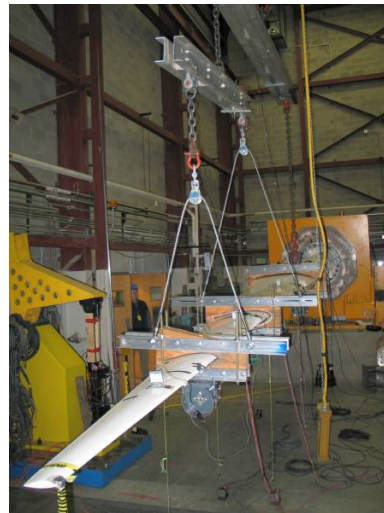
Fig. 13. TX-100 Static Testing
