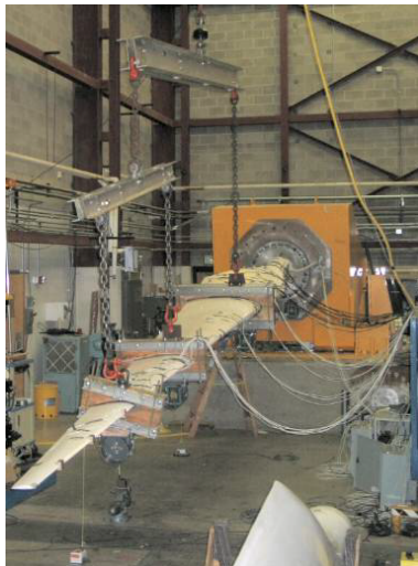
Fig. 12. CX-100 Static Testing
