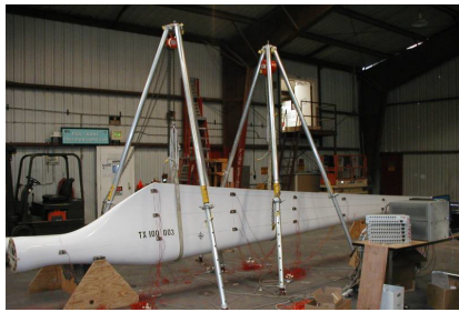
Fig. 10. Modal Test Set-up
