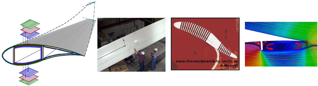
Fig. 5a, 5b, 5c, 5d. Bend-twist Coupling, Aileron, Airfoils with Changing Shape, Microtabs
