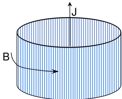
$J \times B$  force implodes wire array, forming a hot, dense plasma on axis
