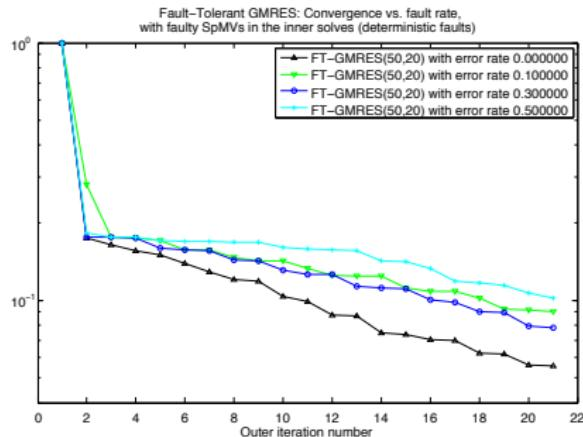
FT-GMRES on III\_Stokes problem, with different fault rates in inner solves' SpMVs.
