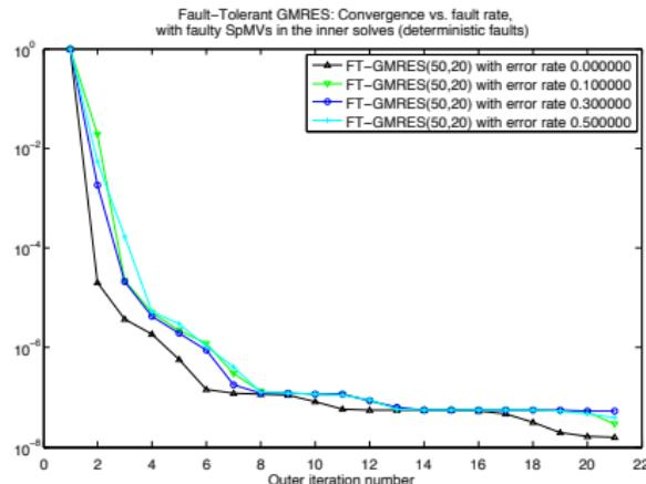
FT-GMRES on mult\_dcop\_03 problem, with different fault rates in inner solves' SpMVs.
