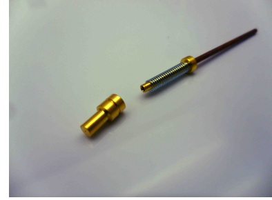
Figure 4: Left: MWPC frame, composed of Noryl, showing the holes for the wire feedthroughs. Right: Spring-loaded wire feedthrough. A wire passes through the hole in the center of the left brass part, through the right brass part and into the copper tube, where it is crimped.
