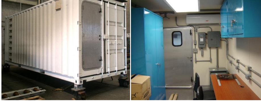
Figure 14: UNOLS-based science van prepared to house operators and data management systems during SNMREC ocean current research turbine testing.
