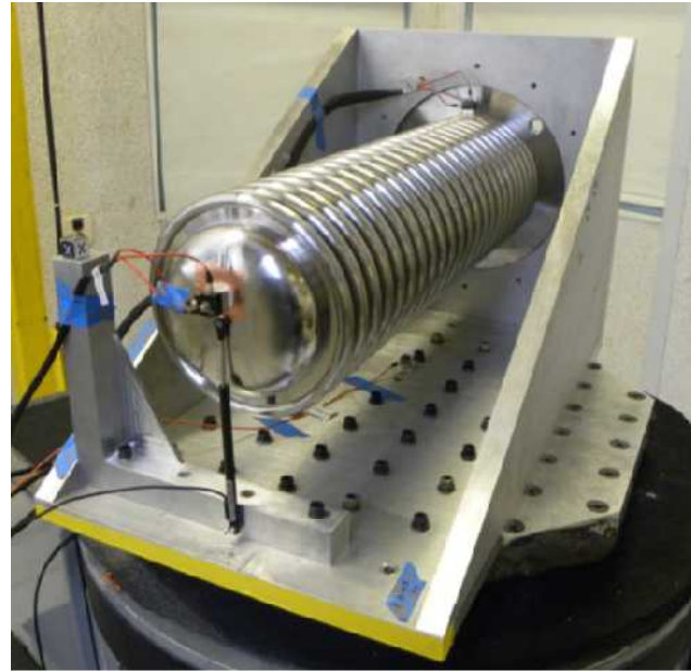
Figure 2. Cascade section of the C1.1 laser-triggered gas switch in a test fixture on the shaker table.
