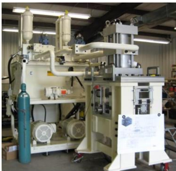
Figure 14. Picture of the “Mold-Press”, designed for foam panel production. The hydraulic system is shown on the left, and the mechanical molding system on the right. The equipment is 12 feet high.
