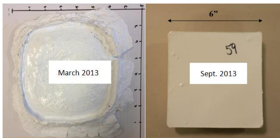
Figure 15. Panel produced by semi-continuous process prior to modification (left) and after modification (right)
