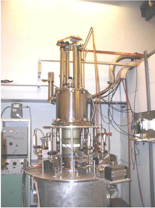
Figure 1. A general view of the 34.3 GHz magnicon.
