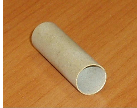
Fig. 14. Small ground pipe made of the same material as the ring shown in Fig. 11, having a wall thickness of 0.6 mm.
