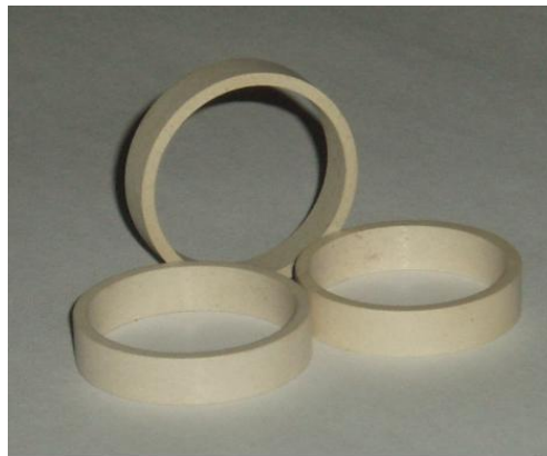
Fig. 12. The ferroelectric ring with a diameter of 34 mm, length 7 mm and thickness of 2 mm.
