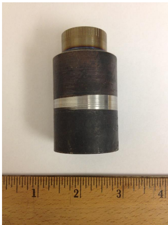
Fig. 2.1. A typical pressure vessel manufactured from two halves cylinders by inertial welding technique.
