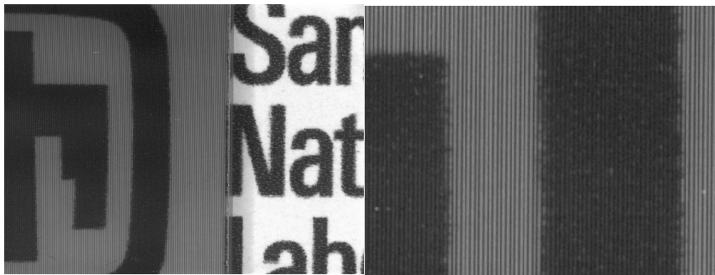
Figure 10. (left) The left-hand side of this image is covered by the die pair patterned with Au lines and brought into registration by the interactions between these lines, which were coated with self-assembled monolayers of dodecanethiol. (right) When the image is magnified, the registered lines can be clearly seen. This image includes the upper right ‘shoulder’ of the thunderbird.
