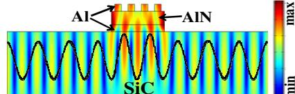
For optimum  $f.Q$  and insertion loss need to maximize energy coupling from the piezoelectric AlN stack to the low loss SiC
