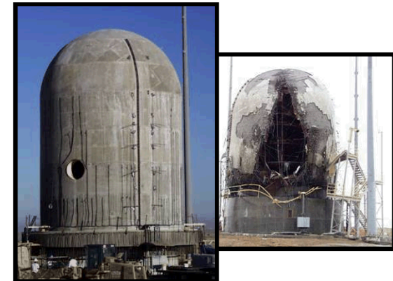
1/4-Scale Prestressed Concrete Containment Vessel Test to Failure (Japan)
