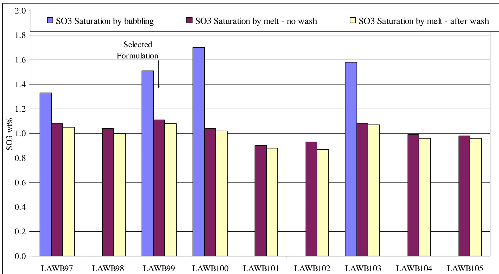
Figure 2.10. Measured sulfate solubility by SO 2 /O 2 gas bubbling and by remelting with excess SO 3 for nine new LAW Envelope B crucible glasses.
