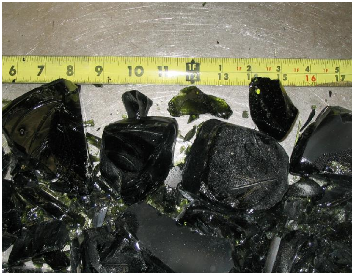
Figure 5.7.b Close-up of glass discharge from end of tests showing small sulfate inclusion (single yellow spot, top right; WVZ-G-11A, 1.15 wt. % SO 3 in feed, additional sugar).
