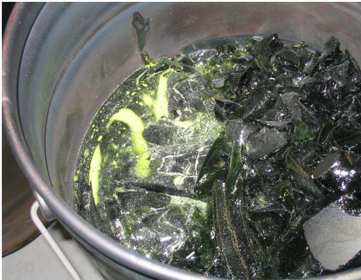
Figure 5.8. Sulfate on surface of discharged glass (WVY-G-155B, 1.15 wt% SO 3 in feed, additional sugar).
