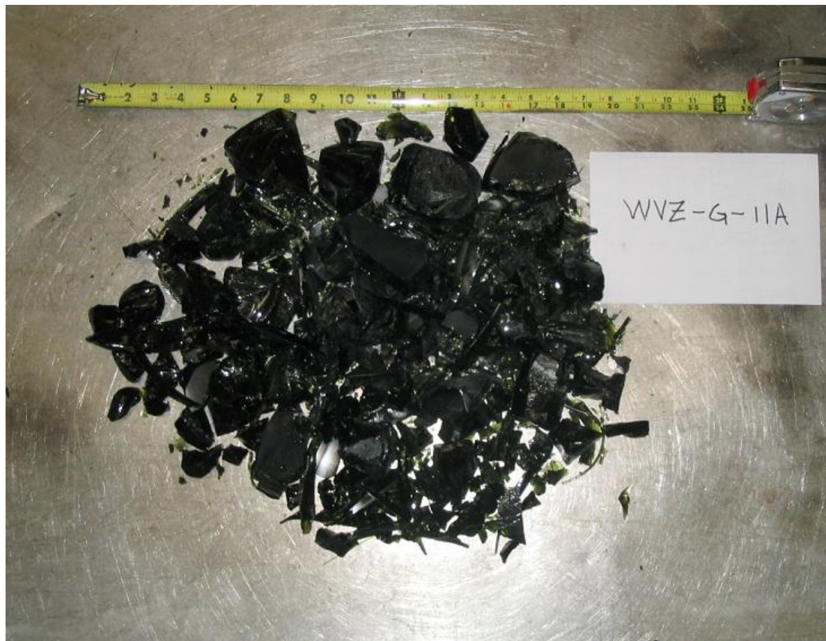
Figure 5.7.a Entire glass discharge from end of tests (WVZ-G-11A, 1.15 wt% SO 3 in feed, additional sugar).
