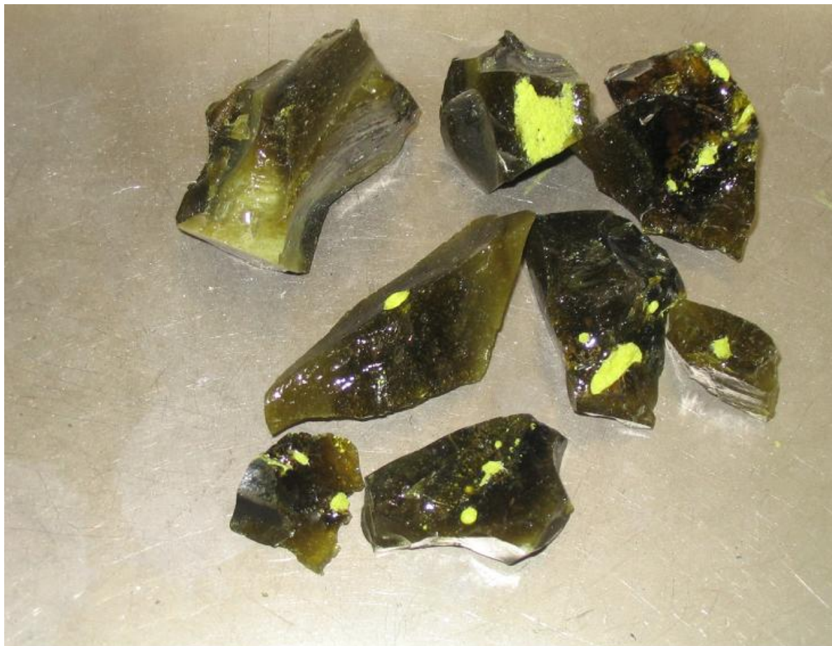
Figure 5.6. Secondary phases in discharged glass (WVY-G-121B/C, 1.3 wt% SO 3 in feed).
