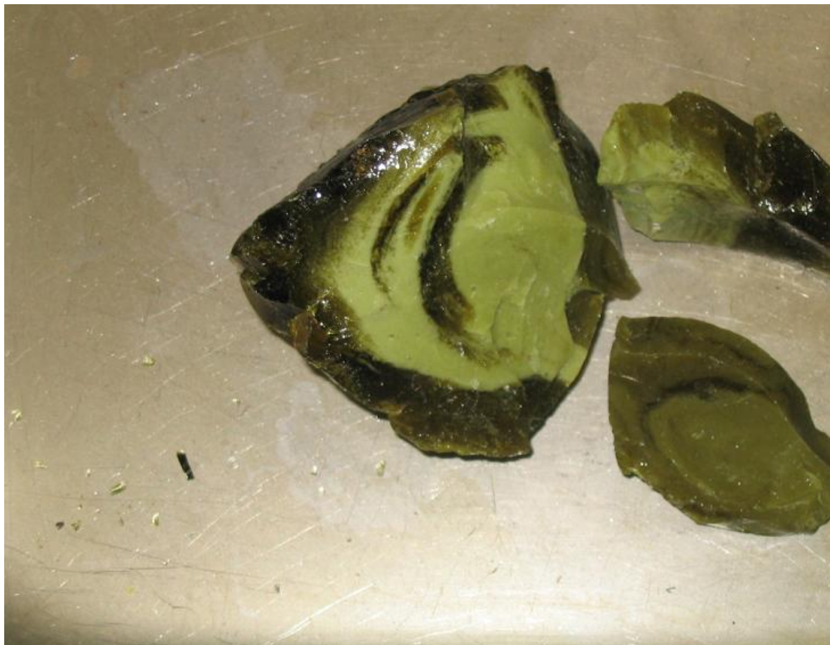
Figure 5.9. Opaque secondary phases in discharged glass (WVY-G-137B, 1.15 wt% SO 3 in feed).
