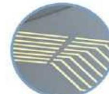
**NICK THE WIRE** A notch in a few interconnects would be almost impossible to detect but would cause eventual mechanical failure as the wire became overloaded.
