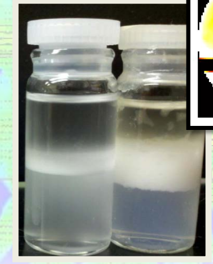
Provided experimental proof-of-concept for use of nanoparticle-stabilized emulsions as a CO 2 leakage deterrent in subsurface flow
