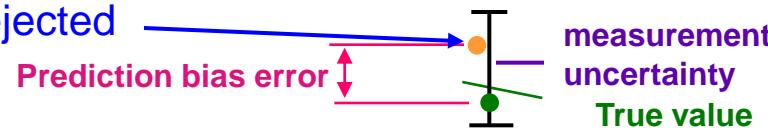
The diagram illustrates a validation test result. A horizontal line represents the measurement. A vertical line segment below it represents the prediction bias error. A vertical line segment to the right of the measurement represents the uncertainty. A green dot at the bottom represents the true value. The text 'measurement', 'uncertainty', and 'True value' are labeled next to their respective components.
