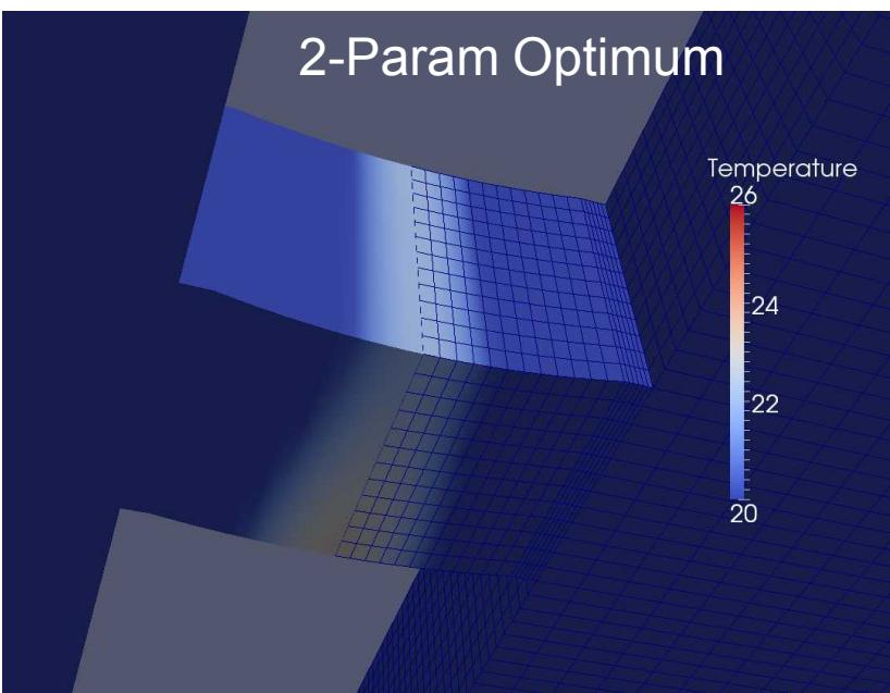
Embedded UQ capability: A UQ Study was performed for the 3D model. PCE expansions are automatically propagated through the PDEs. The full stochastic nonlinear system is solved with Newton's Methods. No application-specific code development was required.
