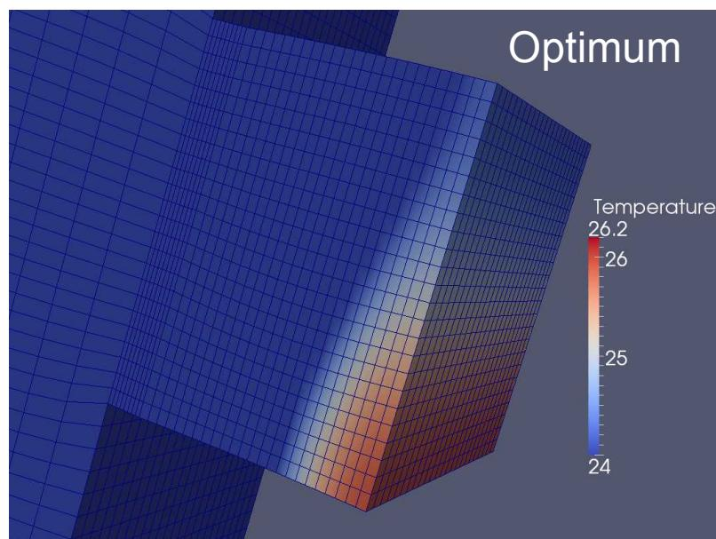
Three parabolic deflections (leading edge, trailing edge, and z-bulge), when subject to a volume constraint on the slider, result in a 2-parameter design optimization. The optimization run results in a significant decrease of  $T_{\max}$
