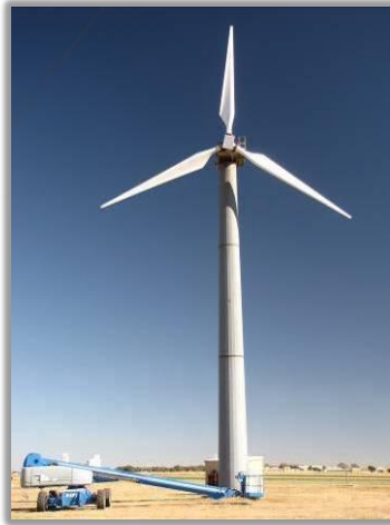
Micon turbine with 9m CX-100 blades
