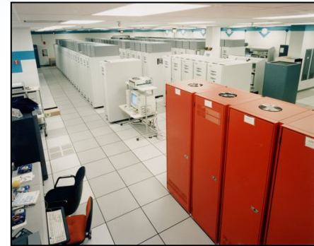
1997 – 1 Teraflop in a room • 2,500 ft 2 & 500,000 Watts
