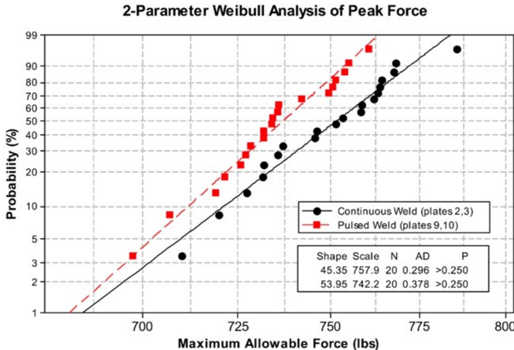
Extrapolating 'pulsed weld' distribution to a low allowable probability of failure:
