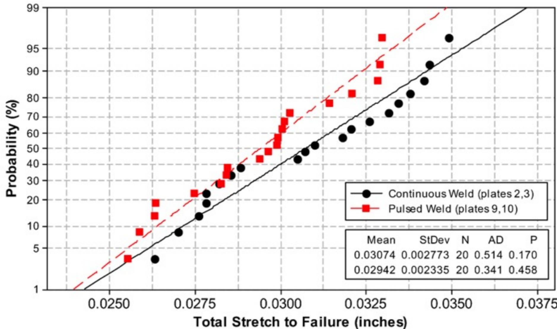
Extrapolating 'continuous weld' distribution to a low allowable stretch:
