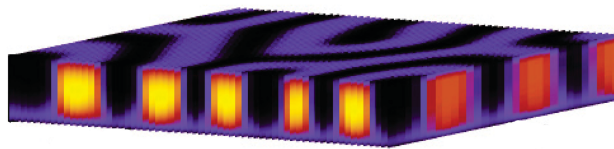
Figure 1. Representative density of A segments in a symmetric mixed brush ( f_A = 0.5 , N_A = N_B ) without lateral confinement. Brush height and lateral box size are set to 3 and 30 R_g , respectively.
